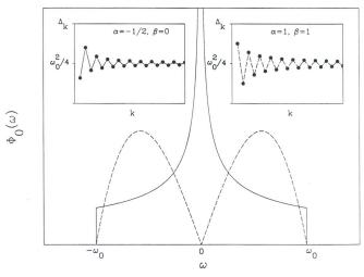
Signature of divergent infrared singularity ( $\alpha < 0$ ): the  $\Delta_{2k+1}$  converge from below and the  $\Delta_{2k}$  from above toward the same limit.
