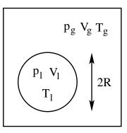
Work done if droplet expands or contracts:  $\delta W = -p_l dV_l - p_g dV_g + \sigma dA$ . Grand potential:  $\Omega(T, V, \mu) = -p_l V_l - p_g V_g + \sigma A$ .
