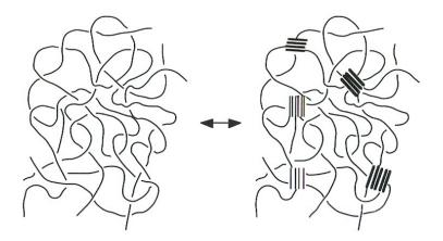
Thermoreversible gelation of long triblock copolymers (with short and identical endblocks) via microphase separation.
