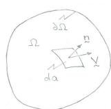
Characterization of the flow of a fluid (in general, compressible) by flux densities of mass, momentum, and energy.
