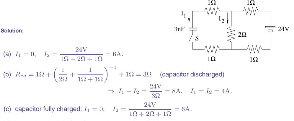
(d) loop rule:  $(2\Omega)(6A) - (1\Omega)(0A) - V - (1\Omega)(0A) = 0 \implies V = 12V.$
