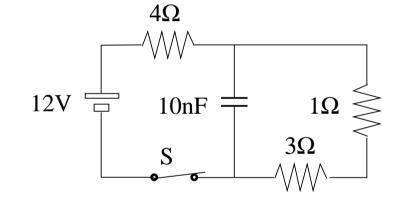
$$I_B = \frac{12V}{3\Omega + 1\Omega + 4\Omega} = 1.5A$$
