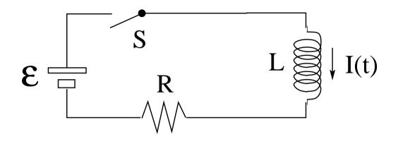
Physical properties of RL circuit during current buildup determined by 3 combinations of the device properties:
