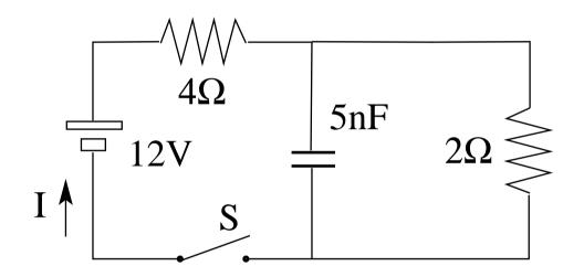
In this RC circuit the switch S is initially open as shown.
