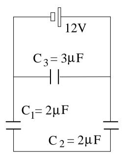
The circuit of capacitors connected to a battery is at equilibrium.
