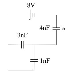
Consider the capacitor circuit shown at equilibrium. (a) Find the equivalent capacitance  $C_{eq}$ . (b) Find the total energy U stored in the three capacitors. (c) Find the voltage  $V_*$  across the capacitor marked by an asterisk. (d) Find the voltage  $V_1$  across the 1nF-capacitor.
