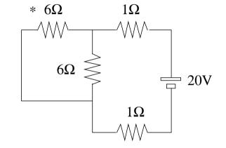
$$R_{eq} = \left(\frac{1}{8\Omega} + \frac{1}{8\Omega}\right)^{-1} + 3\Omega + 3\Omega = 10\Omega \qquad R_{eq} = \left(\frac{1}{6\Omega} + \frac{1}{6\Omega}\right)^{-1} + 1\Omega + 1\Omega = 5\Omega$$
