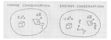
Energy conservation is equally well established. Consider a region of space with electric and magnetic fields and with ideal sources. Electromagnetic energy is carried by the electric field  $\mathbf{E}(\mathbf{x}, t)$  and the magnetic field  $\mathbf{B}(\mathbf{x}, t)$ .
