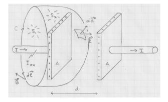
In the setup shown a capacitor is being charged up by a conduction current I flowing in both connecting wires. No conduction current flows between the plates, but an electric field is being built up.
