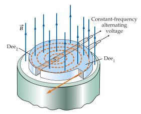
This design only works for non-relativistic speeds:  $v \ll c$ . For particles with relativistic speeds,  $v \leq c$ , the period T depends on v.
