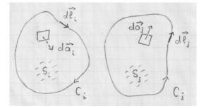
Each loop generates a magnetic field everywhere in that region. The field strength is proportional to the current in the loop.
