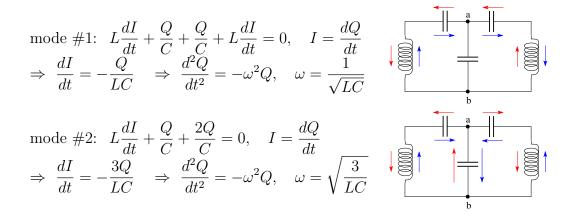
The mechanical analogue of this oscillator consists of two masses connected by three springs as shown. When this system oscillates in the slower mode, both masses move in the same direction all the time and the spring in the middle does not change its extension. The faster mode, by contrast, has the two masses move in opposite direction all the time, which now also compresses and stretches the spring in the middle.
