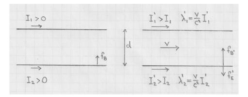
▷ Magnetic field of rail 1 at position of rail 2 and (attractive) magnetic force (per unit length) on rail 2 when both rails are at rest:
